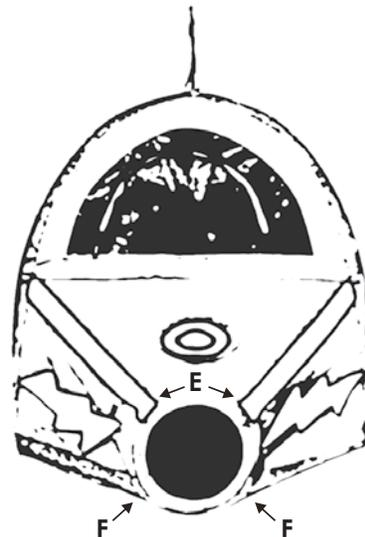
Insert the 2 Grey G3 poles (**F**) into the pole sleeves on each side of the front of the structure on the bottom of the nose.
